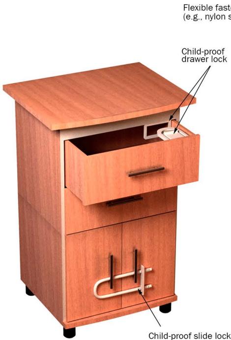
Figure E. Securing cabinet doors and drawers.
